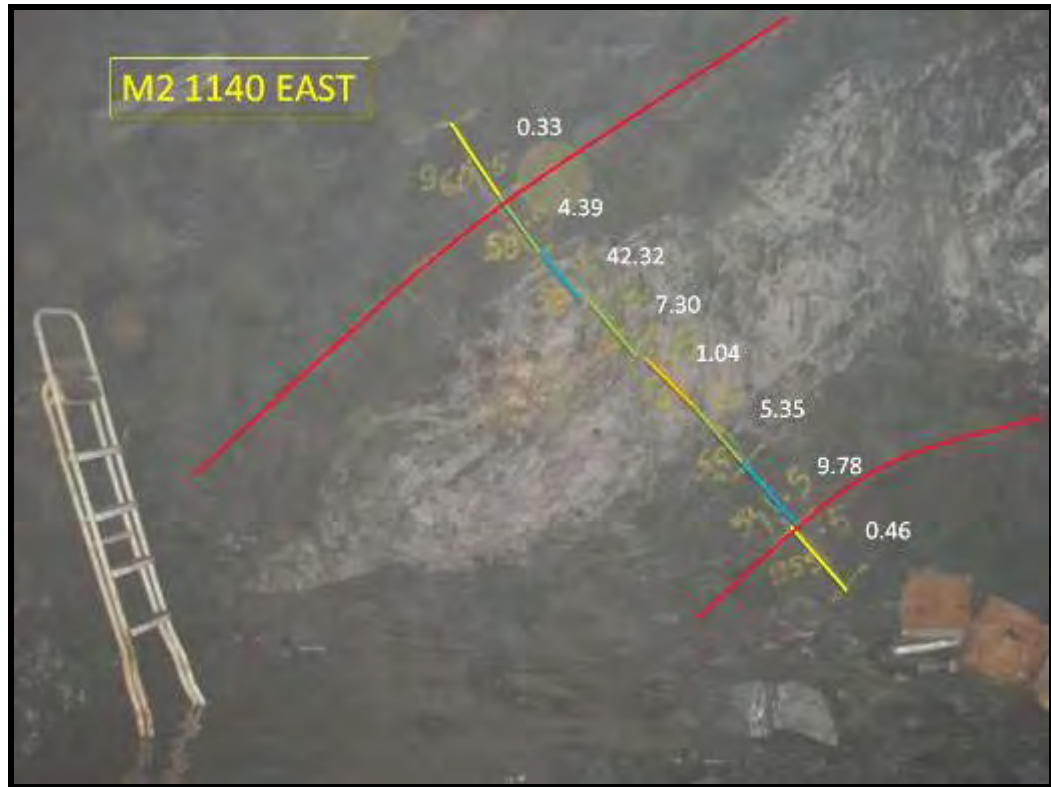
Photo #1: Channel Sampling on M2 Lode (1140 East drive). Channel Sample Average Grade of 3m at 10.86g/t gold.
